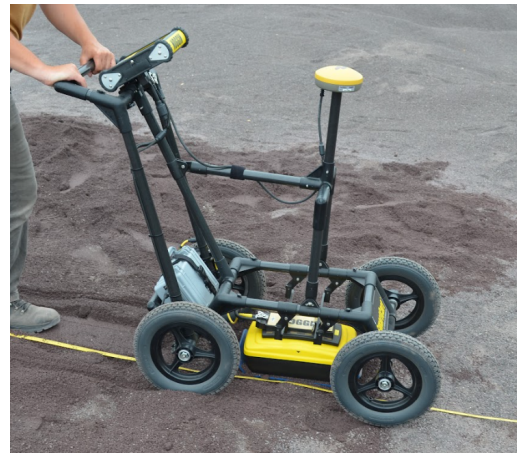
Figure 2: NOGIN® 500 MHz GPR antenna attached to Sensors and Software SmartCart
